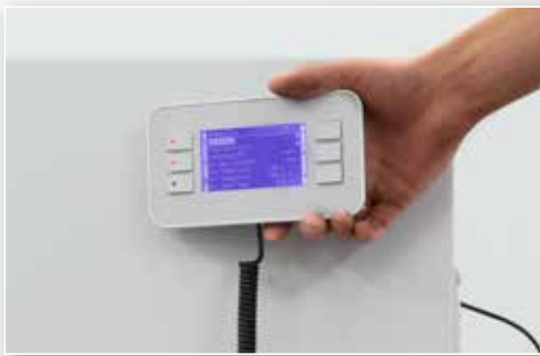
Magnetic control unit for free placement
