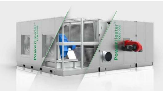
**The redesigne**d Power Heater enables a highly efficient hop drying together with resource-conserving operation. **The heart** of the device is the combustion chamber. The challenge to be met is an optimal exploitation of the combustion space and the side areas. That's exactly what is achieved by the cone-shaped body, assuring an even firing performance. **Fans** of energy efficiency class IE3 with pressure stable freewheel and backward curved blades.
